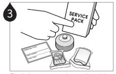
Check the grease pouch capacity and the service pack items (battery pack, grease pouch & dust cover).
