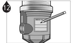
Note the installation date and the scheduled completion date of lube cycle on the lubricator using the label provided in the Service Pack for maintenance purposes.
